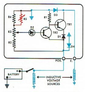
through ground into the regulator, and then through diode D3 back to the field winding. Note that the diode blocks current flow from the battery and generator output terminal to ground.
