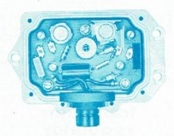
There are many different models of transistor regulators, each designed to meet the requirements of a specific application. Although the external appearance of these regulators may vary considerably, the internal circuitry on each model is basically the same. Since this section describes the basic internal circuit, it applies equally well to all models of transistor regulators.
