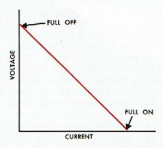
On some models of regulators it is desirable to assist the zener diode in reducing to a minimum the length of time needed for the transistors to switch from "on" to "off" and from "off" to "on." By reducing this time factor the heat developed in the transistors is decreased. To explain why this is true, consider the accompanying illustration.
