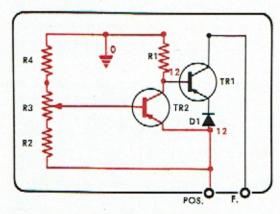
In this illustration, a back-bias diode D1, a driver transistor TR2, and a series of resistors R2, R3, and R4 have been added to the circuit. Since the base of transistor TR2 is connected to ground through resistors R4 and a portion of R3, this transistor will turn "full on," and emitter-collector current will flow through resistor R1 to ground. The potential on the collector of TR2, neglecting the small drop in the transistor, will be 12 volts.
