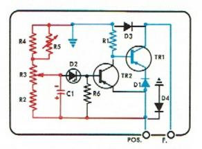
Since the resistance of transistors decreases with increases in temperature, it is possible at higher temperatures for a small leakage current to flow through the emitter-collector of transistor TR2 even though the zener diode completely blocks emitter-base current. This leakage current would cause more heating in transistor TR2, leading to more leakage current and eventually to regulator damage. To prevent this, resistor R6 is connected across the emitter-base of the transistor.
