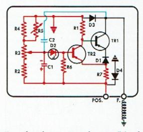
To explain the operation of resistor R7 and capacitor C2, consider the instant of time at which the voltage across the zener diode D2 is 8 volts, and the zener diode starts to conduct current. The driver transistor TR2 and output transistor TR1 can be made to switch more quickly if the voltage across the zener diode could suddenly be increased slightly, say to 8.2 volts. This would cause the zener diode to conduct instantly, and the two transistors to switch instantly.
