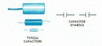
A capacitor, sometimes called a condenser, is a device in which electricity is stored. A capacitor consists of two metallic conductors separated by an insulating material. This often takes the form of thin metallic foil separated by thin paper; the foil and paper are then rolled into a cylindrical shape for compactness.
