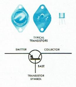
The transistor is a semiconductor that consists of two diodes "back to back," or two diodes sharing a common base material. In the symbol shown, the emitter-base junction represents one diode, and the collector-base junction the second diode. Current flows through the emitter in the direction of the arrow; hence the positive side of a battery is connected to the emitter, and the negative side to the base and collector, as shown. The symbol shown represents a PNP transistor.
