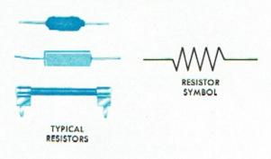
$$\begin{array}{c} \text{AMPERES} = \frac{\text{VOLTS}}{\text{OHMS}} \\ \text{or VOLTS} = \text{AMPERES X OHMS} \\ \text{or OHMS} = \frac{\text{VOLTS}}{\text{AMPERES}} \end{array}$$
