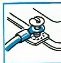
POOR OR LOOSE CONNECTIONS
