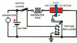
there is no transistor base current, and no collector current will flow. Consequently, the transistor "shuts off" the generator field current and the generator voltage decreases. This causes a decreased pull in the regulator shunt winding which allows the contacts to reclose and the cycle then repeats many times per second.
