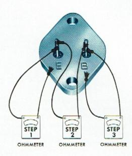
zero, the transistor is shorted. Then connect the ohmmeter as shown in Step 2, and then reverse the connections. If both readings are zero, the diode is shorted. If both readings are infinite, the diode is open. Follow the same procedure for Step 3 as for Step 2.
