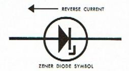
rent in the reverse direction without damage if proper circuit design is used. The zener diode symbol is shown.
