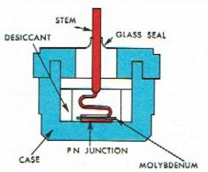
cur. Since moisture adversely affects semiconductor material, a desiccant is located inside the case to absorb any moisture that might enter. Also, a glass seal is used around the diode stem, or lead, to prevent the entry of moisture.
