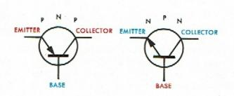
conventional current flow; that is, from positive to negative in the external circuit. As previously described, it is convenient to look upon current flow in the PNP transistor as a movement of holes, and in the NPN transistor as a movement of electrons. Although the electrons move against the arrow in the NPN transistor, this is not contradictory as it is easier to visualize the current carriers (electrons) as being emitted by the emitter into the base and collector.
