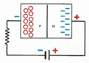
there will be no current flow. In effect, a very high electrical resistance is created at the junction area. This type of battery connection is referred to as reverse bias, which causes the diode to block current flow.
