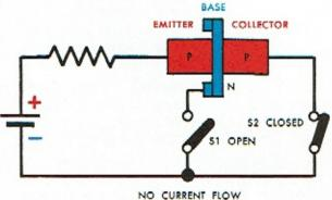
An important observation is that with switch S2 closed and switch S1 open, no appreciable current will flow. The reason for this is that with the base circuit open, there are no holes being injected into the base from the emitter, and consequently there are no holes in the base which can be attracted by the negative
