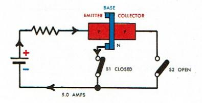
At this point in our discussion, it is well to recall a definition of current flow — the movement of electrons from atom to atom in a conductor. Under this definition, the electrons in this circuit flow from the negative battery terminal through the base-emitter back to the positive side of the battery. However, in order to better understand the operation of a PNP transistor, it is necessary to accept hole movement as a theory of current flow, and to apply this theory to the PNP transistor.
