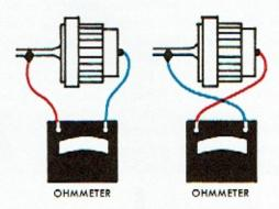
It is important to observe that a diode cannot be condemned because two ohmmeters give different readings on the diode. This occurs due to the different internal resistances of the ohmmeters and the different states of charge of the ohmmeter batteries. Since each ohmmeter will send a different current through the diode, the two resistance values read on the meters will not be the same. This is borne out by the non-linear voltage-current
