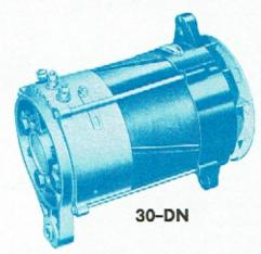
Shown in the illustration is a 30-DN Series generator used in truck, marine, industrial, and other heavy-duty applications where a high output at idle is required. This type of essembly has mounting lug spacing to meet specific requirements, an external fan for cooling, and on some models, fully enclosed dual brush sets.
