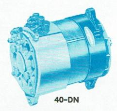
A generator in the 40-DN Series designed for automotive, truck, marine and industrial applications having high electrical loads is shown. This type of assembly uses a 12-pole rotor similar to the 14-pole type, and either a "Y"- or a delta-connected stator. The diodes are of the threaded type, and some models have fully enclosed dual brush sets.
