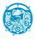
With a 14-pole rotor having strong magnetic fields, a stator containing many turns of wire, and adequate cooling, the generator is a high output source of electricity.
