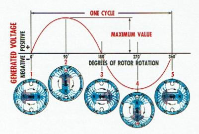
Pictured in the illustration are different positions of the rotor as it rotates at constant speed. In the top portion of the illustration is a curve showing the magnitude of the voltage which is generated in the loop of wire as the rotor revolves.
