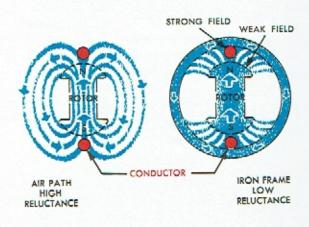
the conductor which lies between the bar magnet and the frame.
