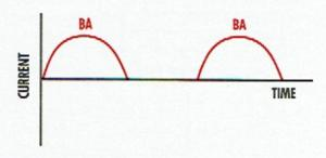
The output is increased when four diodes are used to provide "full wave rectification." Note that the current is more continuous than with one diode, but that the current varies from a maximum value to a zero value. It is particularly important to observe that the current flow through the external load resistor is in one direction only. The A. C. voltage and
