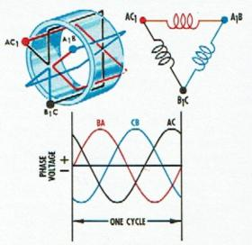
When the ends of the loops of wire marked A<sub>1</sub>, B<sub>1</sub> and C<sub>1</sub> are connected to the ends marked B, C and A respectively, as illustrated, a basic three phase "delta"-connected stator is formed. The three A. C. voltages available from the delta-connected stator are identical to the three voltages previously discussed, and may now be denoted as the volt-
