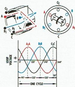
With the rotor making 60 complete turns in one second, there will be 60 such curves, one coming right after the other, resulting in 60 cycles per second. The number of cycles per second is called the frequency. Since the generator speed varies in automotive type applications, the frequency also varies.
