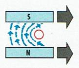
The direction of current flow is determined by the direction of the magnetic lines of force and the direction of motion of the magnetic field with respect to the conductor. To visualize this, note the illustration, where magnetic pole pieces are being moved so that the magnetic lines of force are cutting across a conductor.
