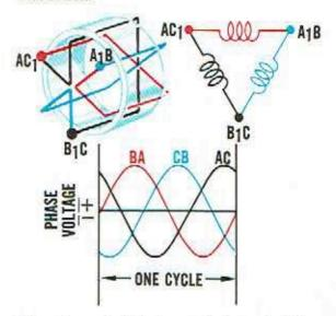
When the ends of the loops of wire marked A<sub>1</sub>, B<sub>1</sub> and C<sub>1</sub> are connected to the ends marked B, C and A respectively, as illustrated, a basic three phase "delta"-connected stator is formed. The three A. C. voltages available from the delta-connected stator are identical to the three voltages previously discussed, and may now be denoted as the voltages from B to A, C
