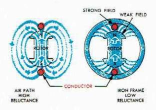
It is important to note that a very large number of magnetic lines of force are at the center of the tip of the magnet, whereas there are only a few lines of force at the leading and trailing edges of the tips. Thus, there is a strong magnetic field at the center and a weak magnetic field at the leading and trailing edges. This condition results when the distance, called the air gap, between the magnet and field frame is greater at the leading and trailing edges than at the center of the magnet.
