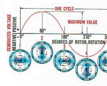
Pictured in the illustration are different positions of the rotor as it rotates at constant speed. In the top portion of the illustration is a curve showing the magnitude of the voltage which is generated in the loop of wire as the rotor revolves.
