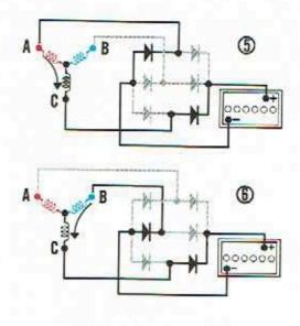
Following the same procedure for periods 3-6, the current flow conditions can be determined, and are shown in the illustrations. These are the six major current flow conditions for a three-phase "Y"-connected stator and rectifier combination.
