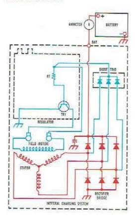
As rotor speed increases, the voltages increase, and current flows from the stator, through the diode trio, R1, the base-emitter of TR1, through the ground circuit, and back to the stator through the grounded diodes in the rectifier bridge. With TR1 turned on, current also flows from the stator through the diode trio, the field, TR1, the ground circuit and the grounded diodes in the rectifier bridge back to the stator.
