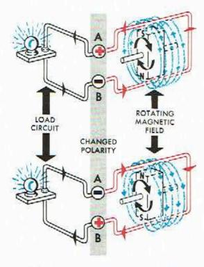
With the magnet rotating as indicated, and with the S pole of the magnet directly under the top portion of the loop and the N pole directly over the bottom portion, the induced voltage, as determined by the Right Hand Rule, will cause current to flow in the circuit in the direction shown. Since current flows from positive to negative through the external or load circuit, the end of the loop of wire marked "A" will be positive (+) polarity and the end marked "B" will be negative (-).
