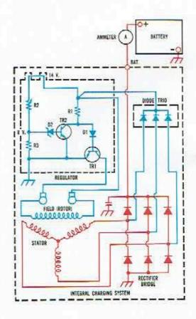
Since zener diode D2 is a special kind of diode that will allow current to flow when the voltage across the diode reaches a certain value, let us assume to illustrate how this diode works, that the Integral Charging System is operating at 14 volts. With 14 volts across R2 and R3, the voltage divides such that 8 volts appears between R2 and R3. This same 8 volts is impressed across D2 and TR2, and we are assuming that 8 volts is the breakdown voltage of D2.
