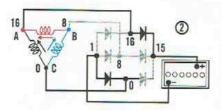
During period 2, the maximum voltage developed is in phase AC, and the voltage potentials are shown on the illustration at the instant the voltage is maximum. Also shown are the other phase voltages, and again, the current flow through the rectifier is identical to that for a "Y" stator, since the voltages across the diodes are the same. However, as during period 1, all three delta phases conduct current as illustrated.
