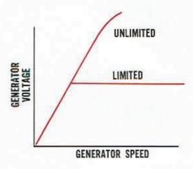
The regulator limits the generator voltage to a preset value by controlling the generator field current. It operates electronically to alternately "turn off" and "turn on" the voltage across the field winding. In a sense, the transistor regulator is nothing more than a very fast acting electronic switch. This switching, between open and closed and back again, can occur at a rate as low as 10 times per second, and as high as 7000 times per second.
