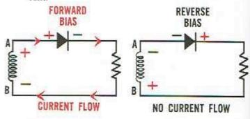
The current flow that would be obtained from this arrangement is illustrated. Since the current flows only half the time, the diode provides what is called "half-wave rectification." A generator having only one diode would provide very limited output.
