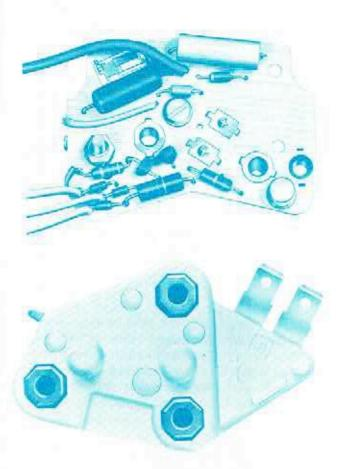
Both types of regulators use the same basic electronic circuit. Since this circuit contains transistors, the regulator is commonly called a transistor regulator.
