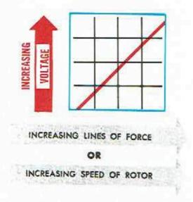
The voltage will also increase if the bar magnet is made to turn faster because the lines of force will be cutting across the wire in a shorter period of time.
