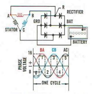
A delta-connected stator wound to provide the same output as a "Y"-connected stator also will provide a smooth voltage and current output when connected to a six-diode rectifier. For convenience, the three-phase A. C. voltage curves obtained from the basic delta connection for one rotor revolution are reproduced here and have been divided into six periods.
