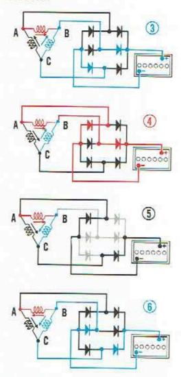
This concludes our study of the fundamental principles by which a simple, basic generator develops three A. C. voltages which are then rectified to a single D. C. voltage and current for use in the electrical system. Although the typical voltage values used in the recent illustrations ignore line drops, they serve very well to show in simplified fashion the sequence and direction of current flow through the stator and diodes.
