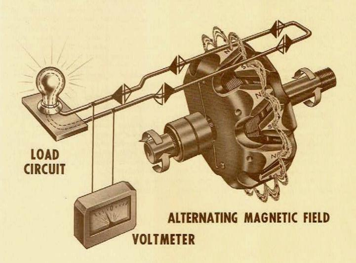
To illustrate further how an alternating voltage is produced, consider a simple two-pole permanent magnet type rotor and a stator that contains a single loop of wire. Only the ends of the loop of wire are shown in the chart.
