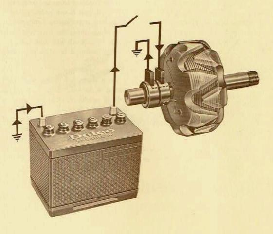
The magnetism created by this field current causes the poles on the rotor to become alternately North and South poles. It will be shown later that this magnetic field is used to produce alternating voltages in the stator windings.
