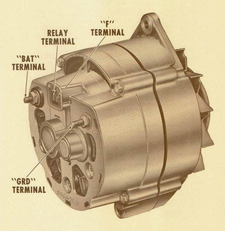
The Delcotron consists primarily of two end frame assemblies, a rotor assembly, and a stator assembly. The rotor assembly is supported in the drive end frame by a ball bearing and in the slip ring end frame by a roller bearing. These bearings are pre-lubricated and therefore do not require periodic lubrication. A grease-filled reservoir in the drive end frame prolongs bearing life. The roller bearing in the slip ring end frame is permanently lubricated prior to assembly into the frame.
